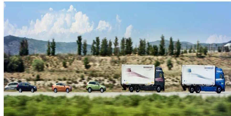
Figure 2. Photo. SARTRE demonstration of three automated cars and one automated truck following the lead truck in a platoon (May 2012).
