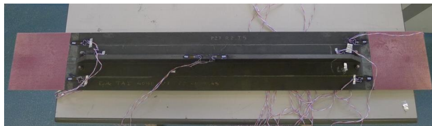
Example of test component in tension
