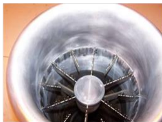
Typical intake measurement rake system
