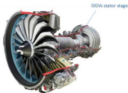
Figure 2 : Outlet guide vanes stator stage (~40 OGVs) in actual engine environment
