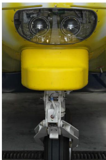
Fig.1 Front landing gear fairing integrated into M28 05 aircraft
