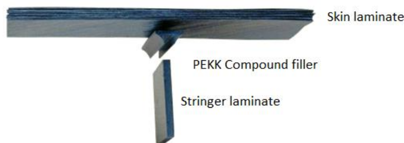
Figure 3. PEKK compound used to join a stringer to a skin (Butt joint)
