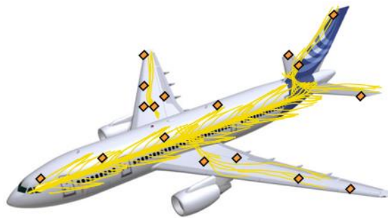
Figure 3 – Potential structural on board health monitoring distribution
