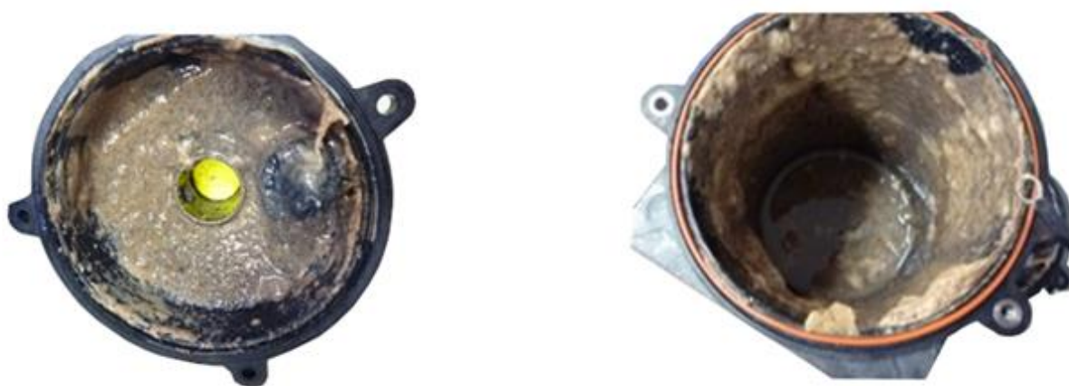
Figure 1: Container with significant biofilm growth due to wet surfaces and presence of organic materials
