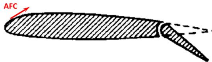
Fig1: Main wing element with installed flow control at the leading edge
