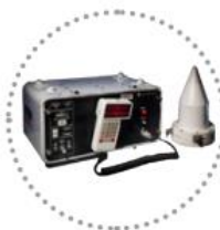
TI-4100 NAVSTAR GPS Receiver, 1981 One of the first commercial GPS receivers.
