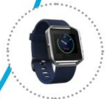
Fitbit Blaze, 2016 One of the most popular wearable devices, which includes GNSS, a heart rate monitor and a battery life of up to one week.
