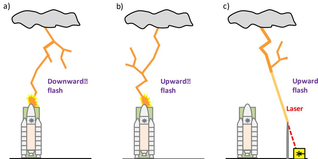
a) Downward lightning to victim; b) upward lightning; c) upward lightning facilitated by laser filamentation discharges the cloud and protects the potential victim.
