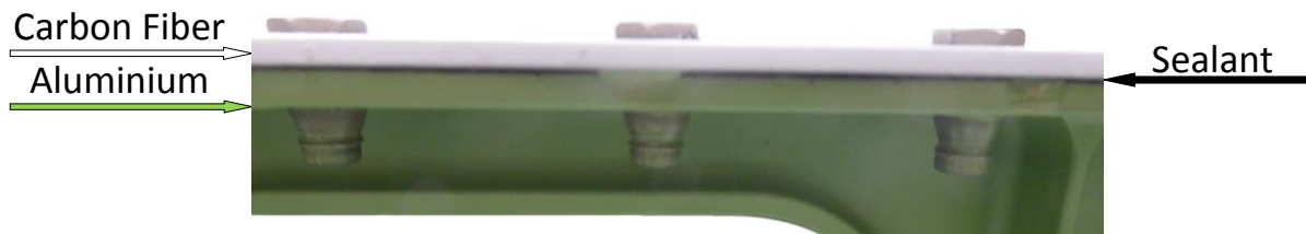
Figure 1. Typical assembly where one way assembly and automated fastening would be preferred
