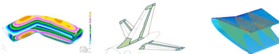
Empennage Fairings Location and DFEM Analysis examples (only as reference)
