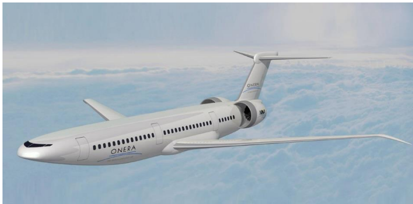
Figure 2 – 180° BLI – ONERA NOVA concept (Wiat, 2016)
