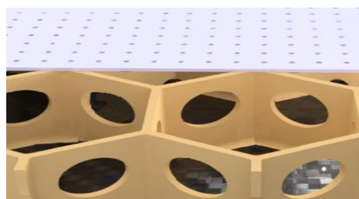
Fig. 3. Schematic view of a honeycomb printed structure underneath the microperforated skin.
