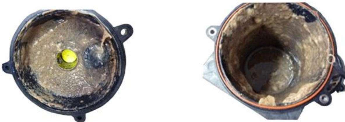
Figure 1: Container with significant biofilm growth due to wet surfaces and presence of organic materials
