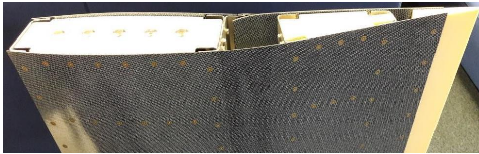
Figure 2: Proof of Concept Winglet morphing TE Flap
