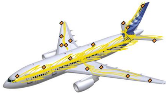
Figure 3 – Potential structural on board health monitoring distribution
