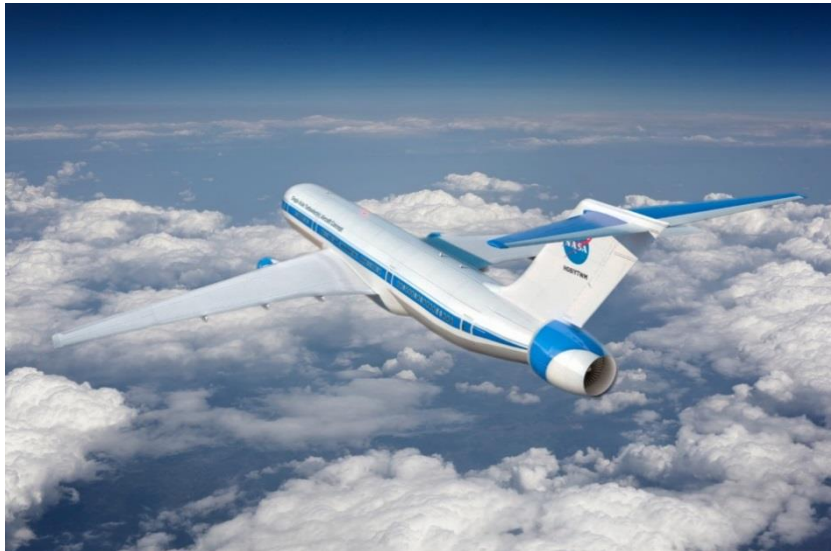
Figure 1 - Propulsive Fuselage – NASA's STARC-ABL turboelectric Plane Concept (Jansen, 2017)
