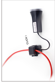
Non-intrusive Power sensors
