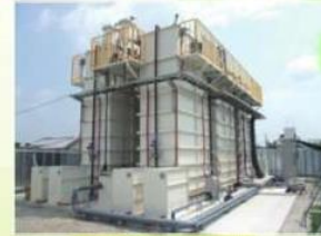
Energy-saving membrane bioreactor pilot test plant
