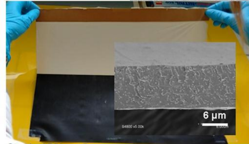
Scaling up of reinforced membrane
